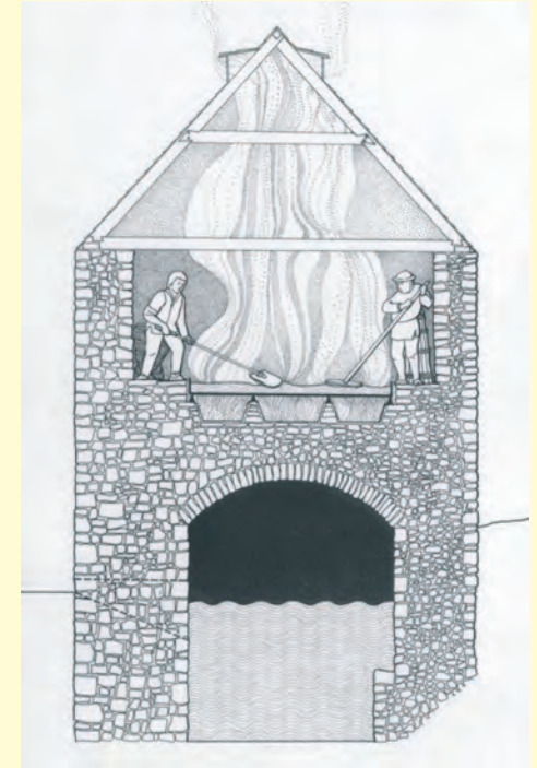
At Port Eynon in Gower, the ruins of an unusual mid-16th century salthouse have been excavated and conserved. Built on the coast by John Lucas the fortified building was altered and extended to become a salt works. It was probably the most technically advanced salt works of its day. Sea water was pumped from the cistern to the heated salt pans above to make the salt.
